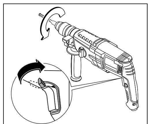
**7. Регулировка глубины сверления / бурения**
