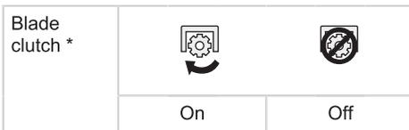
The blade clutch allows the cutter blade to be engaged and disengaged while the motor is running.
